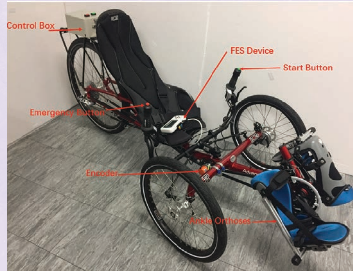
Figure 7. The overall structure of the cycling system including customized seat with seat-raiser, encoder, and ankle orthoses
